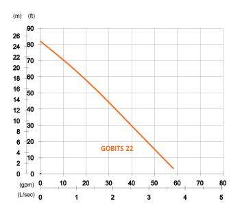
Shaft Speed : 2850 rpm
